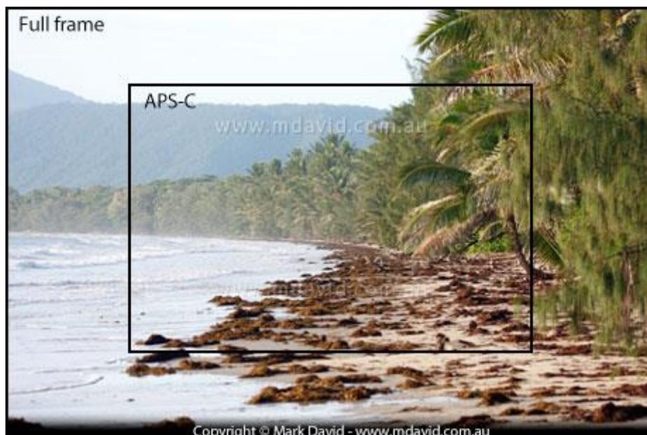
*An APS-C sensor cuts off some of the edges of a scene, compared with a full-frame sensor*
