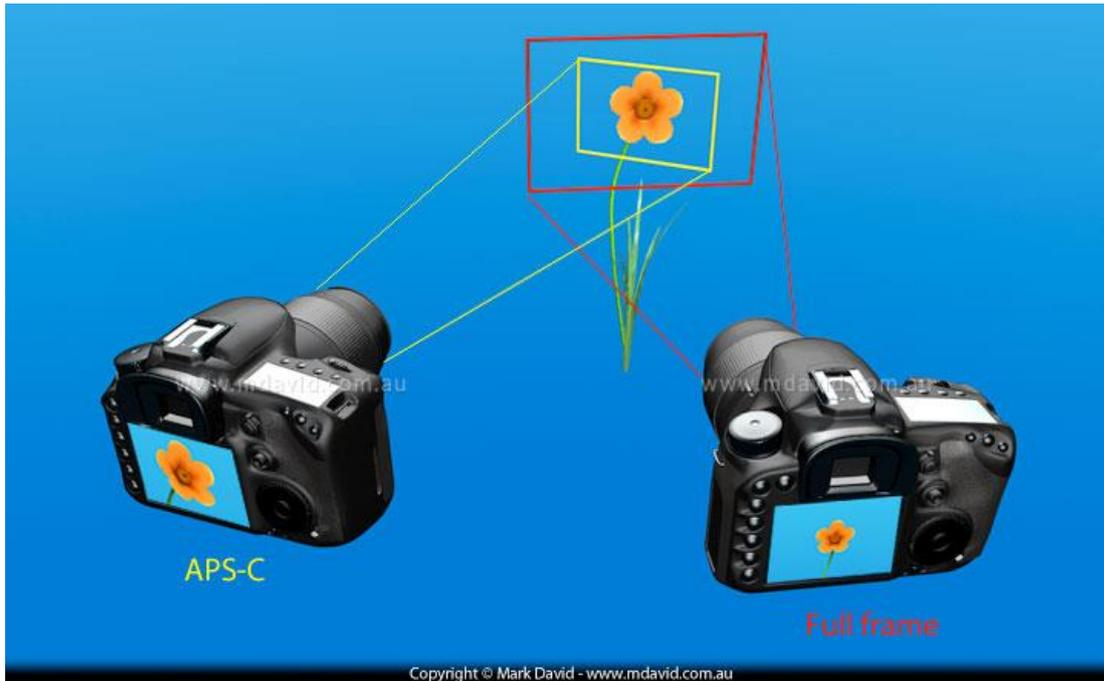
*An APS-C camera and a full-frame camera with identical lenses would see different amounts of the same scene.*
