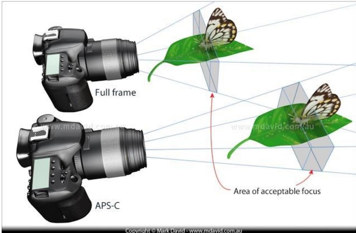
Above: Depth of field increases as you move further away from your subject. This can give an APS-C camera an advantage when taking macro photos because they fill the frame with your subject from a greater distance. Note that this graphic is not drawn precisely to scale.
